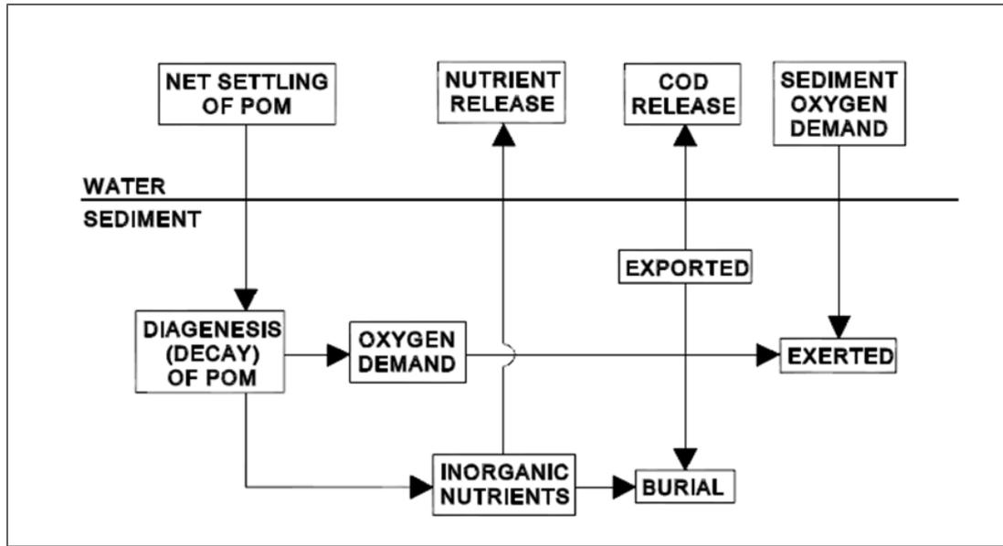
**Figure 3-6 Schematic Overview of Sediment Diagenesis Model Processes (from Park et al, 1995)**
