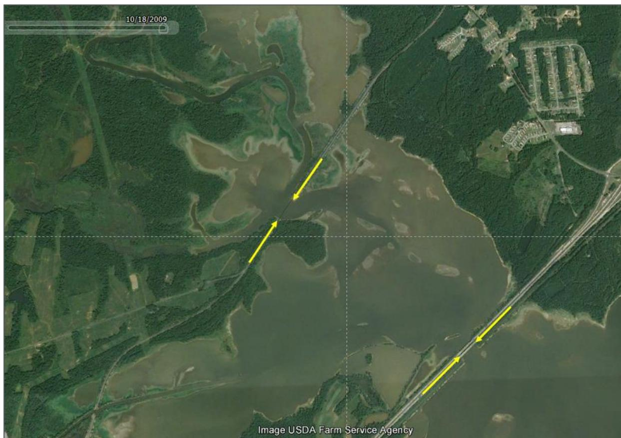
**Figure 3-5 Two Flow Restrictions Caused by Bridge Causeways in Upper Falls Lake**
